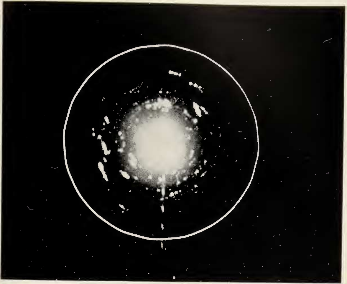
FIG. 4. Enlargement of a 16-mm-radar-film frame (1-minute exposure) showing presentation on radar indicator with antenna on 30^\circ (above horizontal) scan. Circle indicates two nautical miles from radar. White center represents radar recovery time and some ground clutter. Distinct white spots and streaks out from center are typical echoes from passerine birds. Streaks show track of a bird flying tangential to the sweep, the bird having been intercepted by the radar beam in several rotations of the antenna. Single white spots are echoes from birds intercepted only once by the radar beam. Altitude of each target is \frac{1}{2} of the range.
